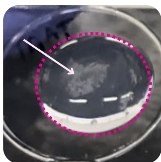
Figure 1. Removable Model embedded in agarose gels. The arrow indicates the Removable Model and the dotted circle shows the agarose gel circumference.
